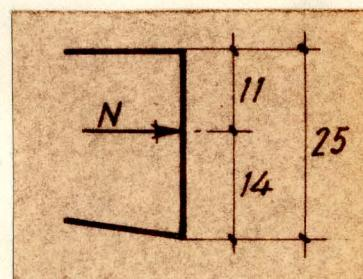
$$\left. \begin{array}{l} \sigma_0 \\ \sigma_1 \end{array} \right\} = - \frac{41,7}{0,25} \pm (2,039 - 41,7 \times 0,015) \times 96 = - 167 \pm 136 = \left. \begin{array}{l} - 31 \text{ N/mm}^2 \\ - 303 \text{ N/mm}^2 \end{array} \right.$$
