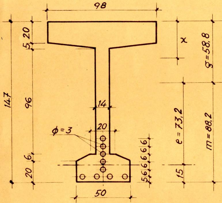
$$A = 98 \times 20 + \frac{98+14}{2} \times 5 + 14 \times 96 + \frac{20+50}{2} \times 6 + 50 \times 20 - 7,1 \times 9 = 4730 \text{ cm}^2 = 0,473 \text{ m}^2$$
