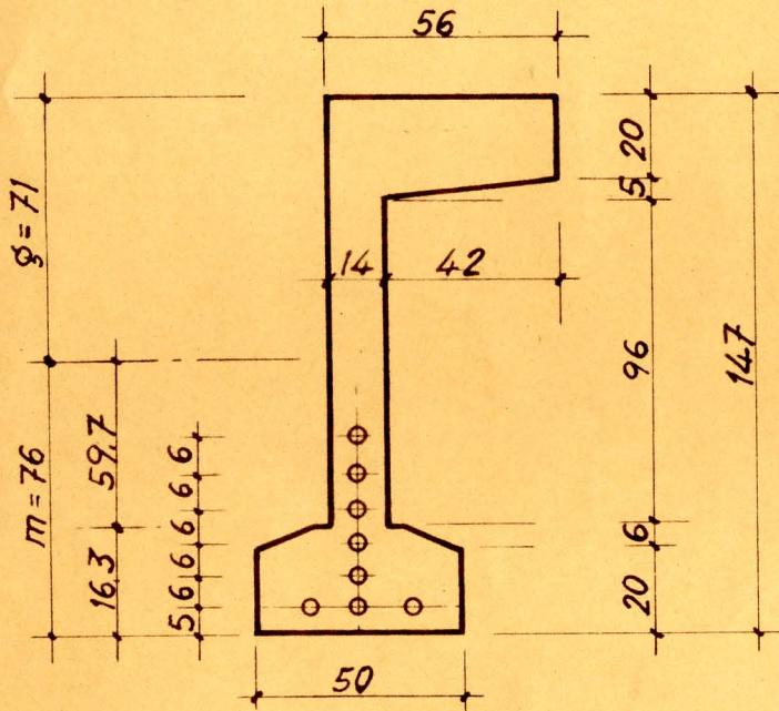
$$A = 42 \times \frac{45}{2} + 14 \times 147 + 26 \times 36 + 6 \times 15 - 71 \times 8 = 3.792 \text{ cm}^2 = 0.3792 \text{ m}^2$$
